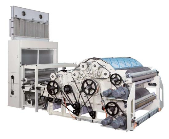
A complete carding section including fiber pre-opener, blend bin, fine opener, hopper feeder, weight pan, carding machine, cross lapper and other peripheral equipment. Taylor made complete carding line according to customer's needs leads to great flexibility of production
