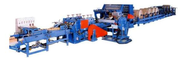
Automatic tubing process produces multi-ply printed Kraft Paper bags in 1 line. Applications of gusset and valve forming available on the same line. Inline flexographic printing from 1 to 4 color.
