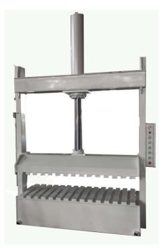
The bale press was specially designed for the packing of woven sack application with easy operation. Finished bales are suitable for domestic or international transportation. Special pressing capacity of bale press can be provided upon request.
