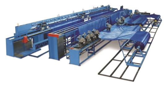
Our automatic tarpaulin making line is designed to weld multiple rolls together with 2 side eyeleting, and cut to desired length simultaneously.
