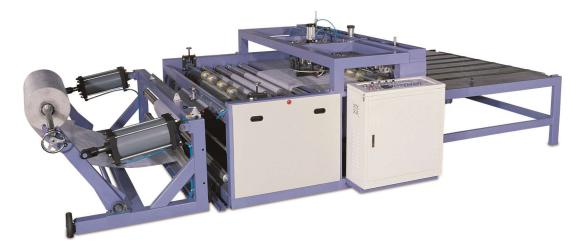
Suitable for converting tubular fabrics and flat fabrics. The FIBC conversion line extends the possibility to produce hoses and bodies used for 1 loop, 2 loop, and 4 loop FIBC. Depends on customer's request, optional O and X punch device available for selection.
