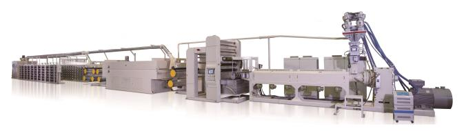
One layer extrusion tape line for PP, or HDPE flat tapes. With melting capacity from 120kg/hour to 700kg/hour, producing films width from 460mm to 1400mm. Tape Winding speed from 250m/min to 450 m/min, which produces premium quality tapes for use in woven sack, Kraft Paper cement sack, PE Tarpaulins, and various applications.
