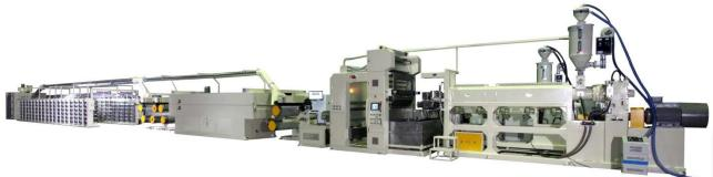
Three layer extrusion tape line with break-through technology to produce 3 layer PP tapes at premium quality and lowest manufacturing costs. The tapes are mainly used for PP woven sack, and various applications.
