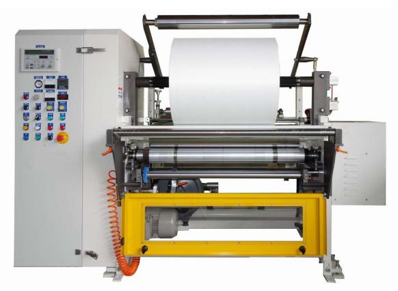
Slitting paper rolls, or laminated woven fabric rolls. Cylinder driven unwinder with optional choice of shaftless unwinder. In-house designed bow roll to avoid over lapping for the finish rolls.
