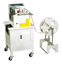
Automatic loop cutting machine for producing carrying belt used for FIBC
