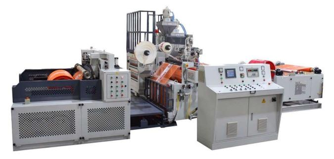
Lamination application designed specifically for label lamination on leno sack. High value added application creates better values and images for our customer.
