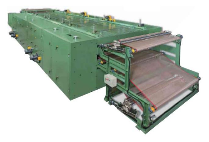
A complete pressing and drying section including heat pressing rollers, oven dryer, embossing rollers, cooling system, accumulator, cutters, winders, and other peripheral equipment. It furnishes the final product with different extent of hardness and touches.
