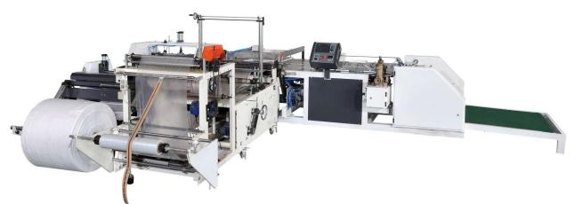
Innovative design for inner liner inserting-cutting-sewing in one process.
